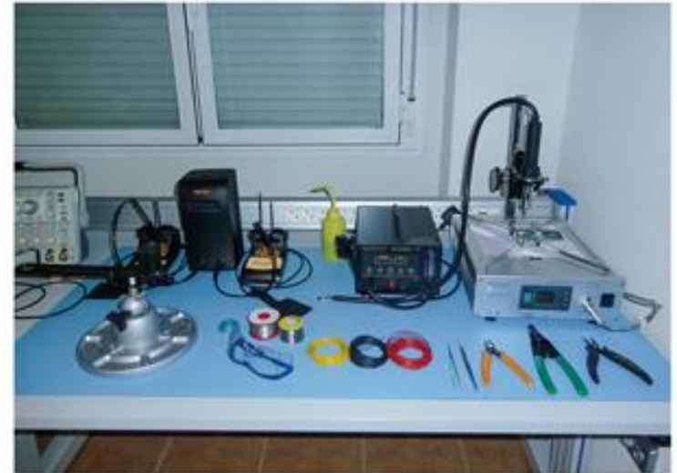
Soldering and hot air reflow
